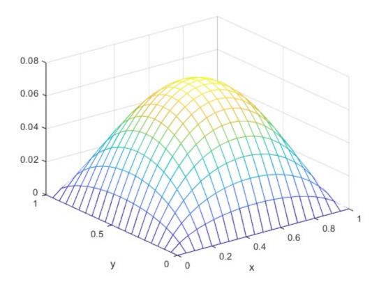
The peak analytical value with 10 terms in the series is 0.0737 and the peak numerical value with 20 division in each direction is 0.0735. This is a relative error of 0.002. If we increase to 40 divisions, the relative error drops to  $5 \times 10^{-4}$ .
