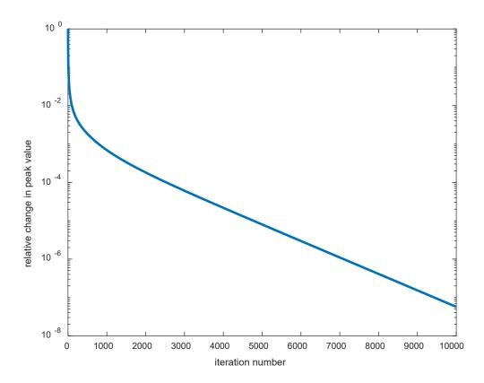
The code will converge faster if we use successive overrelaxation, which increases the change from step to step by a constant. In other words, whereas our previous iteration algorithm can be thought of as
